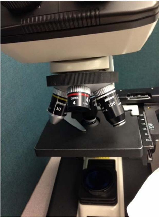
Nikon Alphaphot 2 microscope with 10x widefield oculars, 4x, 10x, 40x and 100x oil immersion objectives, non-removable mechanical stages, abbe condensers, and built-in light source.
